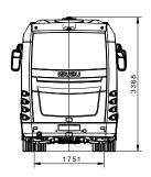
Anadolu Isuzu's 9,5 meter medium-coach, Visigo, has Euro 6 Cummins engine which produces 244 HP at 2100 rpm. The new Visigo provides a comfortable journey to the driver and the passengers with its stylish interior and exterior design, and comfort equipments.
