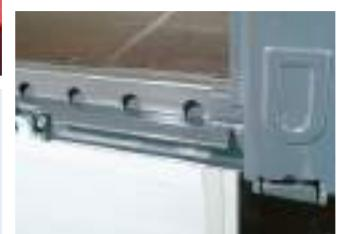
A solid side impact protection avoids damage to the drop sides.
