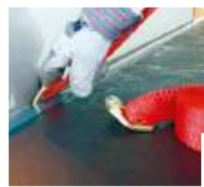
Tension straps with flat hooks allow using the Multi Lock side ravel even when the drop sides are closed.
