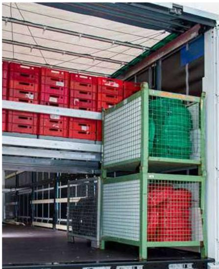
The double deck includes 12 side double bars with an integrated lock rail for side to side. 23 side to side double deck bars are included. This results 33 pallet storage spaces in the second level with the capacity of max. 320 kg per pallet.
