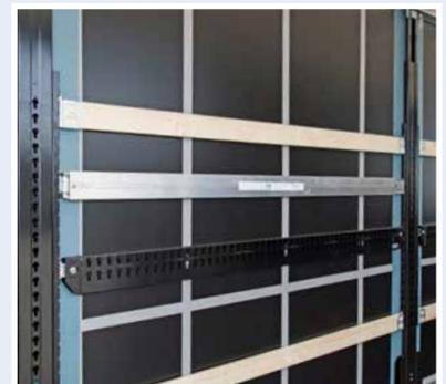
5 pairs of side posts split the platform in 6 fields (5x approx. 2.280 mm and 1 approx. 1.076mm, at the back). In case of non-use, the double deck bars can also be used as "planks" and be stored alongside between the side posts.
