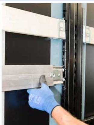
The bars could be adjusted in 100mm steps, from 750-1950mm above the floor.
